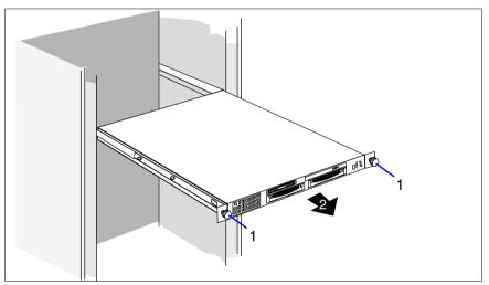
Figure 2: Removing the server
